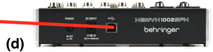
USB Connection From The Mixer-(d) To The USB Port Of The Computer-(a)
