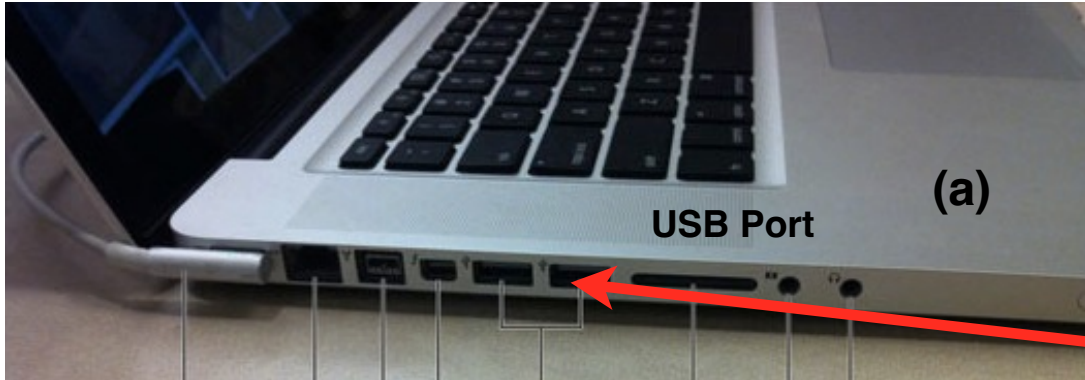
USB Connection From The Mixer-(d) To The USB Port Of The Computer-(a)
