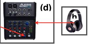
8) You should connect from your audio playback device-(i) using what ever audio connection is needed from your phone or tablet split to 2 mono 1/4" cables-(m) into the line in 3/4 L/R input channels of your
